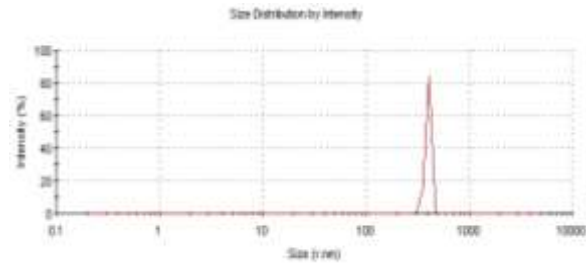
Figure 2 - Fractional composition of nanodiamond particles
